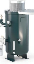
The supersized oil separator design features a larger separation area that reduce the pressure drop during the air/oil separation while providing better filtration, thus making the compressed air system more efficient.
