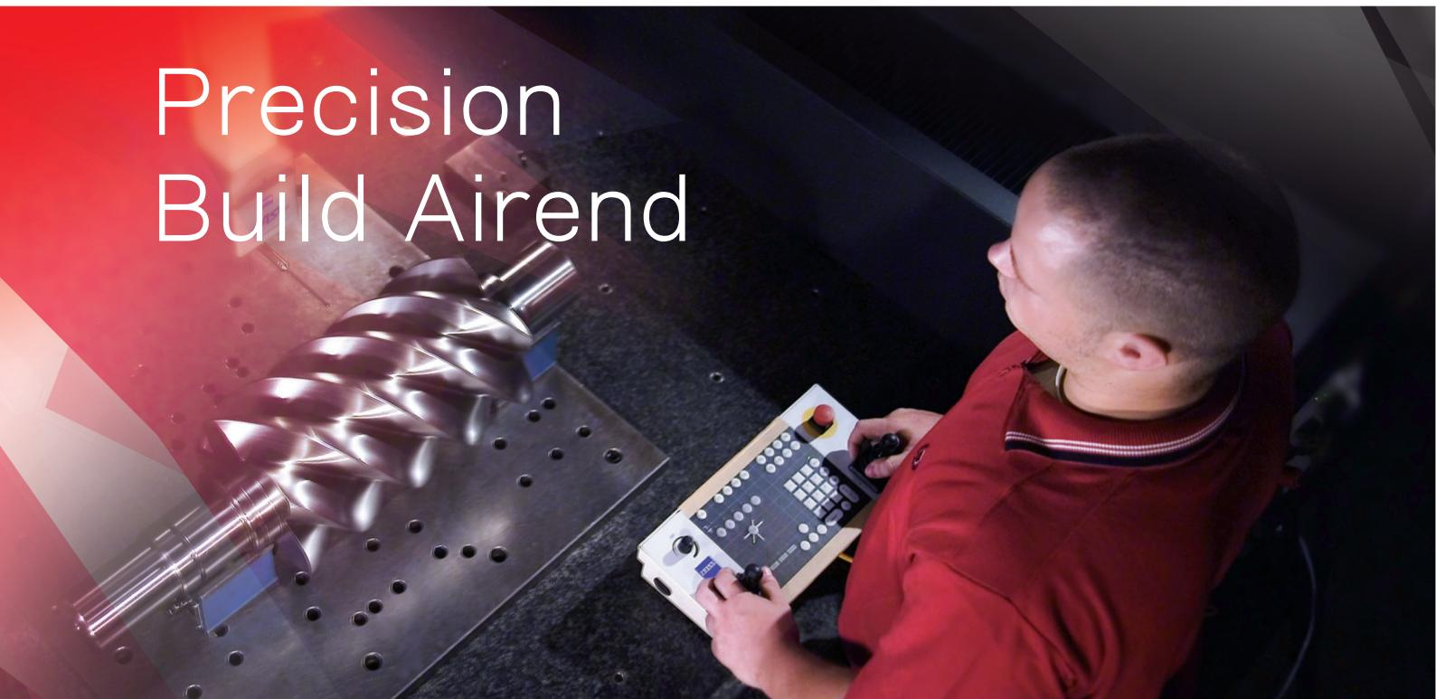
Every Fusheng air compressor incorporates components of the highest quality. From the smallest airend to the largest, each features the latest in rotor profile architecture, combined with multiple roller and angular bearings. Our confidence in the durability and integrity of our design to withstand the radial and thrust forces generated by the compression process, is reflected by our industry-leading airend warranty.
